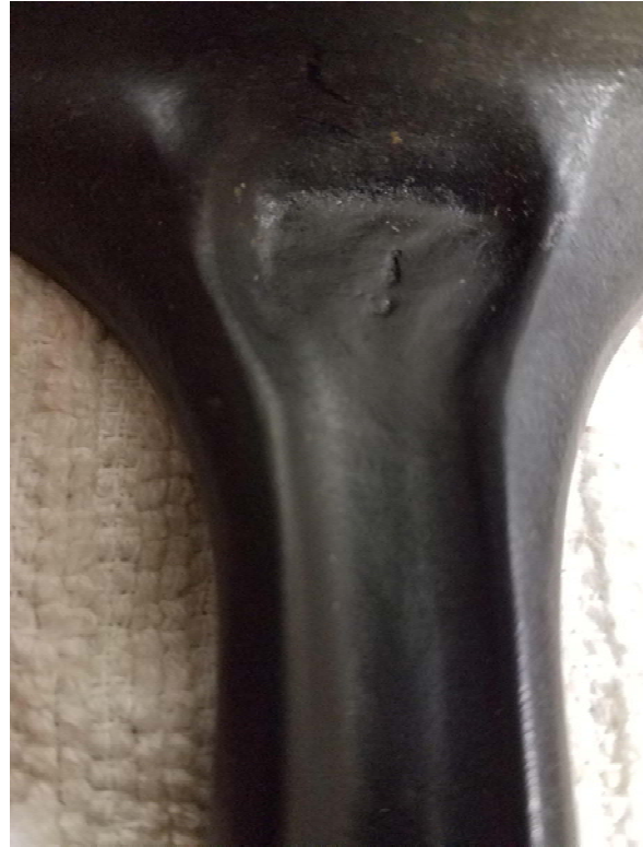
Figure 4. Smooth handle and casting flaw in grooved handle
